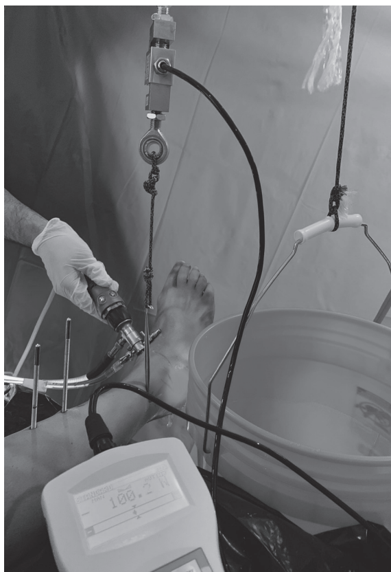
Arthroscopic syndesmotic assessment of right-sided cadaveric specimen. Using an electronic goniometer, a standardized 100N posterior to anterior directed force is applied to the distal fibula via the electronic force gauge.
